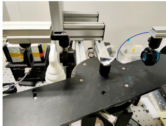
Figure 8 :Optical bench for angular transmission measurements with a white light.
